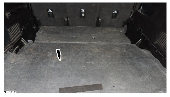
c. Remove the push pins and remove the driver side loadspace trim panel.
