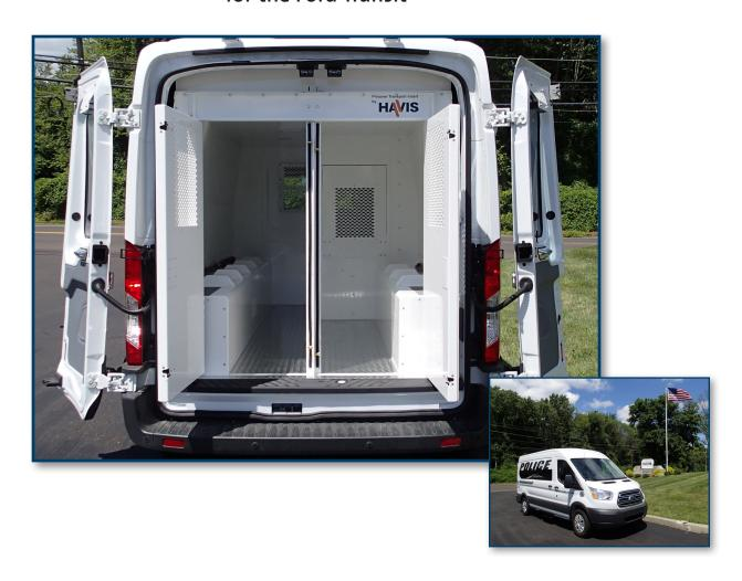
Havis Kwik-Kit® transport systems easily convert cargo and passenger vans into heavy-duty inmate transports while ensuring officer and passenger safety. Offered in three different lengths and one to three compartment options, these units not only help transport people but can also be used for evidence or storage.
