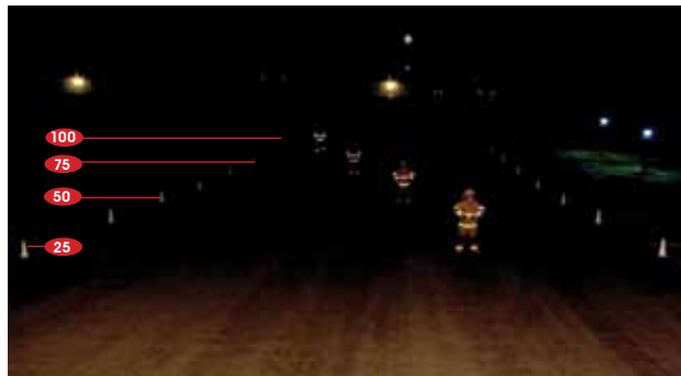
Quartz Halogen Single Lamp @ 100' (150w - 13amp)
