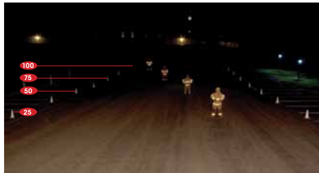
Quartz Halogen Single Lamp @ 100' (300w - 24amp)
