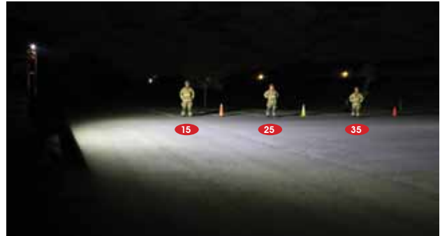
Pioneer Surface Mount - Single - 5° X 90° Flood/Spotlight -PROFILE SHOT (76w - 6amp - 8000 Lumens)
